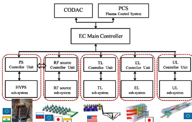
Fig.1. Control architecture of ITER EC system
