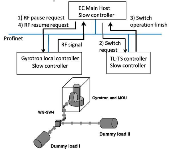
Fig.3. Schematic of TL test stand and control sequence.
