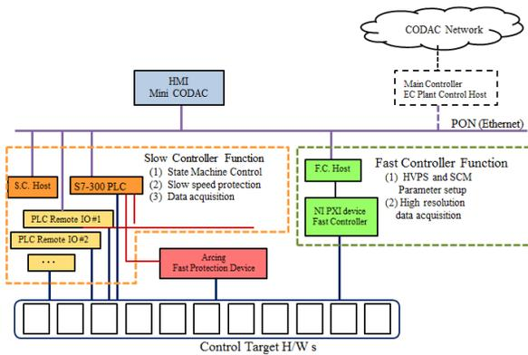
Fig.2. Architecture of Gyrotron Local Controller
