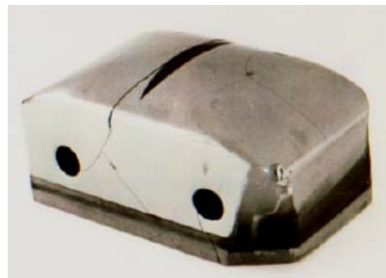
Fig. 1 Broken W test limiter owing to unintentional usage below DBTT
