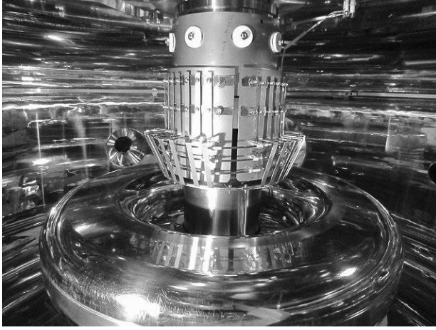
Fig.2. Photograph of the test antenna and the floating coil. About 2/3 part of the antenna is faraday-shielded.
