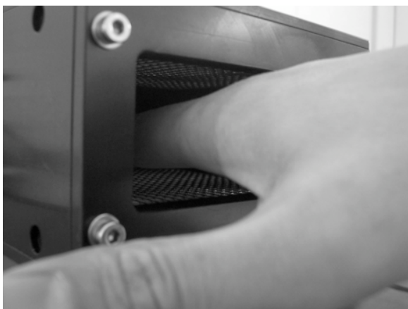
Figure 2. Plasma device for sanitation. Two plasma electrodes are equipped.
