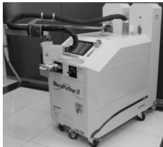
Figure 1. Clinical device for wound treatment. At the end of flexible arm, the plasma torch is placed.
