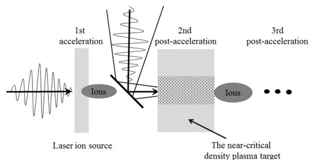
Fig.1. Ion post acceleration scheme and the near-critical density hydrogen plasma target. The near-critical density plasma booster target provides a stable inductive acceleration field, as a post acceleration of laser produced ions.
