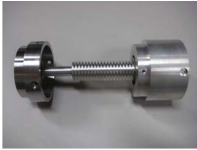
Fig.2. Cylindrical corrugation with both sides propped by supporters.
