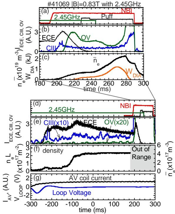
Fig. 1. Time evolution of plasma parameters obtained in NBI startup plasmas (standard config.).
