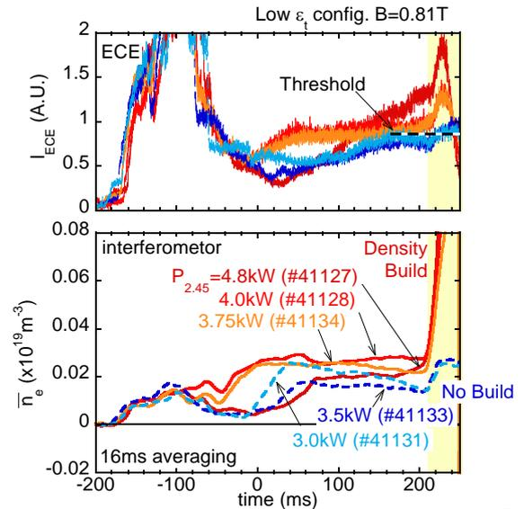
Fig.2. Time evolution of ECE intensity and  $n_e$  obtained in a low toroidicity ( $\epsilon_r$ ) configuration by changing microwave power.
