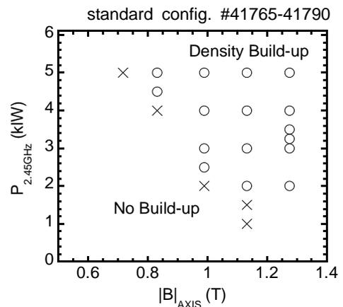
Fig. 3. Relation of density build-up by NBI between microwave power and magnetic field strength.
