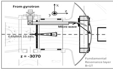
Fig. 2. The side view of the c-ECRH antenna system.
