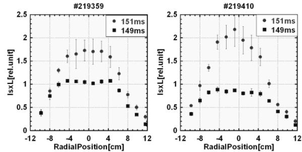
Fig. 5. The radial IsxL distribution at immediately before (149ms) and after (151ms) the c-ECRH.
