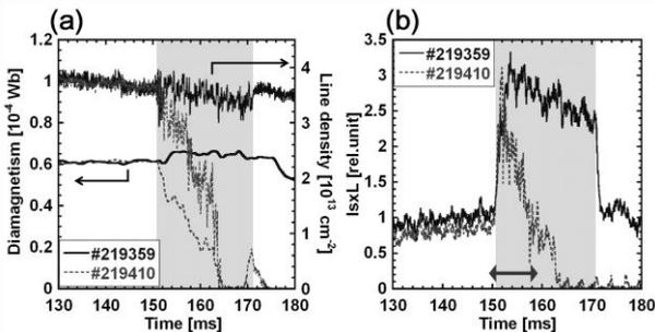
Fig. 3. The time evolution of (a) Diamagnetism, Line density and (b) IsxL. The c-ECRH is injected at shaded region.
