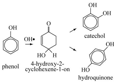
Fig. 1. Decomposition process of phenol when Ar is used as a background gas.
