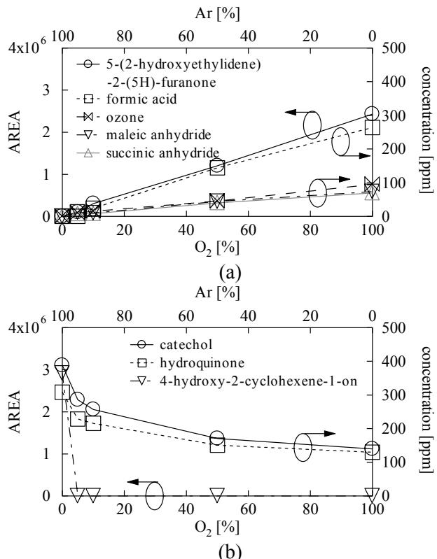
Fig. 3. Concentration of  $O_3$  and by-products as functions of mixture ratio of  $Ar-O_2$
