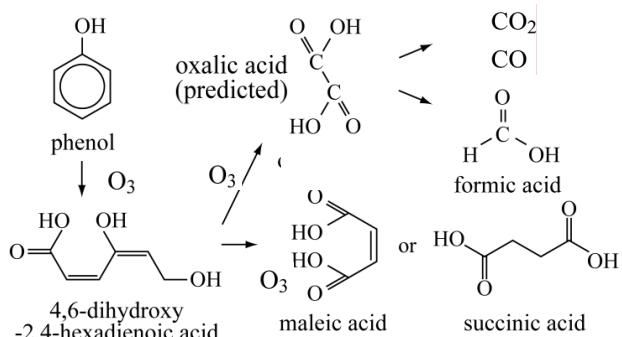
Fig. 2. Decomposition process of phenol when  $O_2$  is used as a background gas
