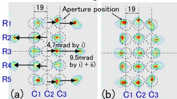
Fig.2. Calculated beam footprints on the target position. (a) Before and (b) after the compensations.
