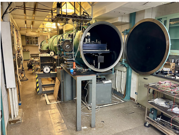
Fig. 1. A 10.7-m Normal Incidence Vacuum Spectrograph providing resolving power \lambda/\delta\lambda \sim 300,000 in the spectral range between 30 and 500 nm.
