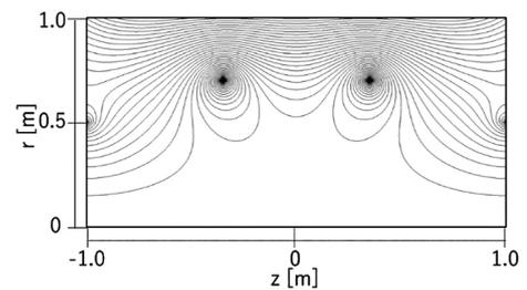
Fig. 2. Contour plot of poloidal magnetic flux.
