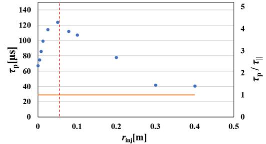
Fig. 4. Particle confinement time  $\tau_p$  (left vertical axis) and its ratio to axial travel time  $\tau_{||}$  (right vertical axis) versus ring injection position  $r_{inj}$ .
