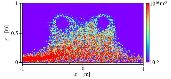
Fig. 3. Color contour of ion density 124  $\mu s$  after particle supply. Here,  $r_{inj} = 0.05$  m.
