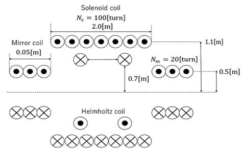
Fig. 1. Coil arrangement diagram in a non-adiabatic trap.
