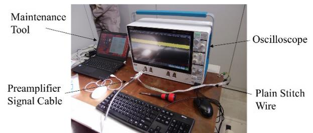
Fig. 6 Photo of the measurement setup. A plain stitch wire for the earthing of the signal earth was used.
