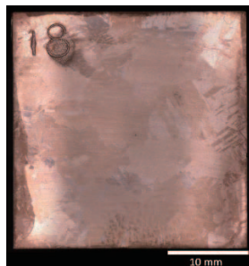
Fig. 3 Grain structure of sample Cu3 with a wide grain size distribution.
