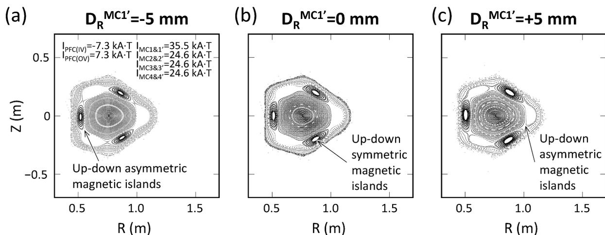
Fig. 9 The calculated magnetic surfaces in the new magnetic configuration to detect the small radial displacements of MC1' by a weighted electric current on the MC1 and MC1'. The calculations with a radial displacement of the modular coil MC1' by  $-5$  mm (a), with no displacement (b), and with a radial displacement of the MC1' by  $+5$  mm are shown.
