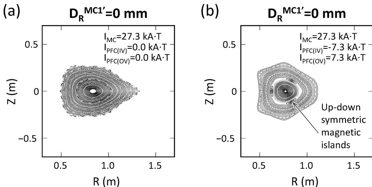
Fig. 2 The calculated magnetic surfaces on the poloidal plane at the fluorescent mesh in a low magnetic field ( $B_t = 0.1 \text{ Tesla}$ ) in the standard magnetic configuration (a) and the specialized magnetic configuration for magnetic surface measurements (b).
