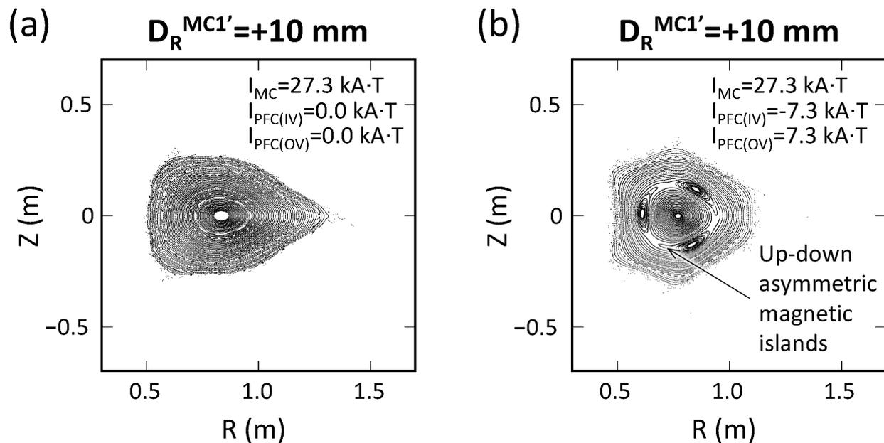
Fig. 4 The calculated magnetic surfaces on the poloidal plane at the fluorescent mesh in the case with a displacement of one modular coil MC1' by +10 mm (outward in the major radius) in the standard magnetic configuration (a) and the specialized magnetic configuration for the magnetic surface measurements (b).
