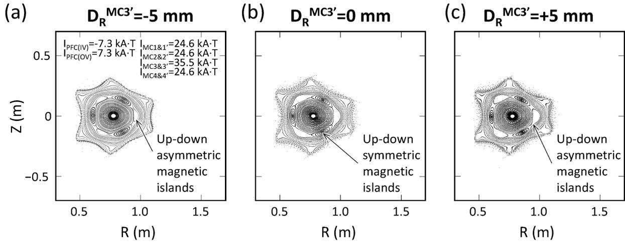
Fig. 10 The calculated magnetic surfaces in the new magnetic configuration to detect the small radial displacements of MC3' by a weighted electric current on the MC3 and MC3'. The calculations with a radial displacement of the modular coil MC3' by  $-5$  mm (a), with no displacement (b), and with a radial displacement of the MC3' by  $+5$  mm are depicted.
