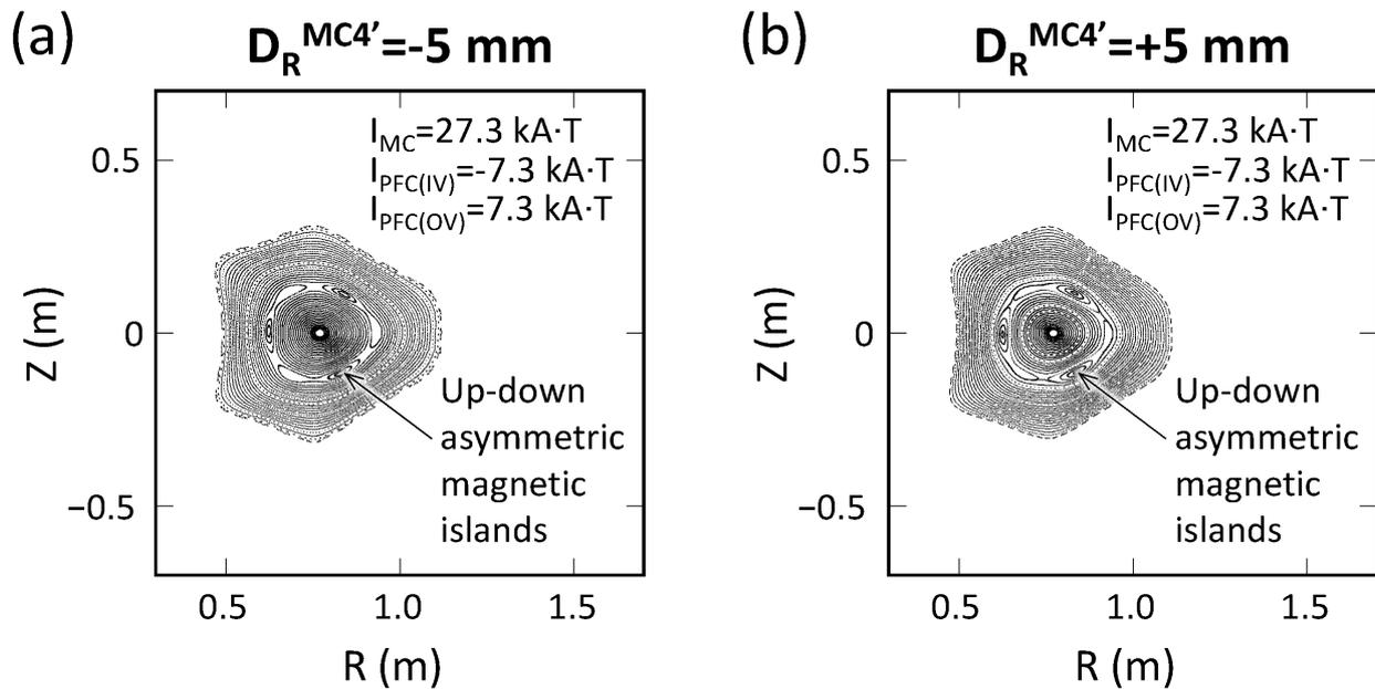
Fig. 8 The calculated magnetic surfaces in the specialized magnetic configuration with radial displacements of one modular coil MC4' by -5 mm (a) and +5 mm (b).
