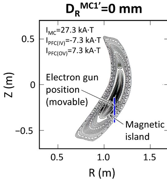
Fig. 3 The poloidal cross-section of the calculated magnetic surfaces in the specialized magnetic configuration for magnetic surface measurements in a low magnetic field ( $B_t = 0.1$  Tesla) at the toroidal position where the electron gun is installed. A solid blue line indicates the positions of the range of the movable electron gun. Only three magnetic islands out of six ones are shown in this figure.
