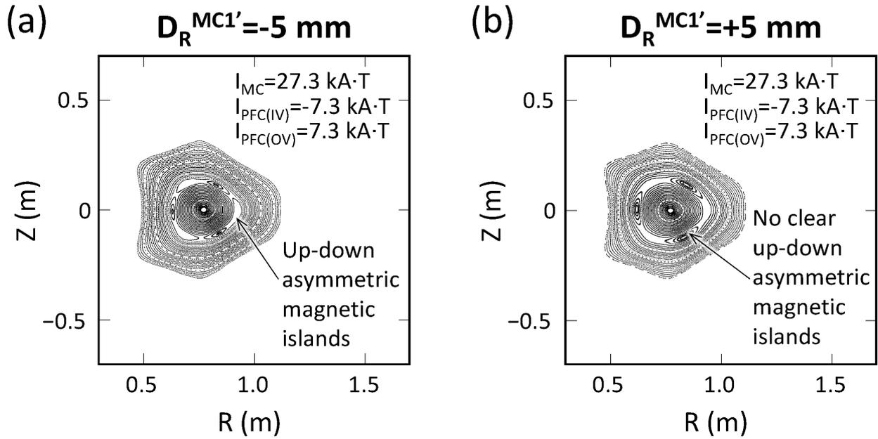
Fig. 5 The calculated magnetic surfaces in the specialized magnetic configuration with radial displacements of one modular coil MC1' by -5 mm (inward in the major radius) (a) and +5 mm (outward) (b).
