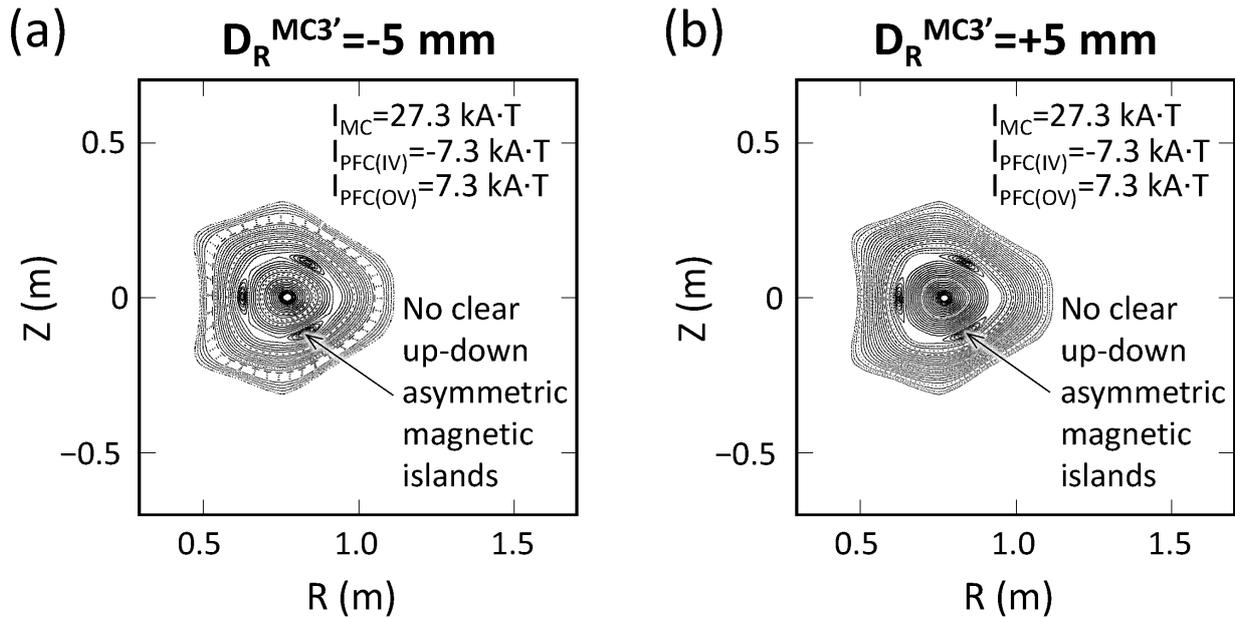
Fig. 7 The calculated magnetic surfaces in the specialized magnetic configuration with radial displacements of one modular coil MC3' by -5 mm (a) and +5 mm (b).
