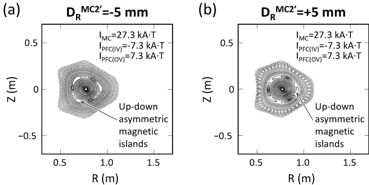
Fig. 6 The calculated magnetic surfaces in the specialized magnetic configuration with radial displacements of one modular coil MC2' by -5 mm (a) and +5 mm (b).
