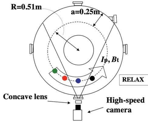
Fig. 1 Experimental setup of the installation of a fast camera onto RELAX from a horizontal port. Solid lines represent the limits of the visual field. A large open arrow indicates the direction of the plasma current  $I_p$  in the plasma core and  $B_t$ . The measurement positions of magnetic probes are indicated by closed color circles, which will be referred to in Fig. 4.
