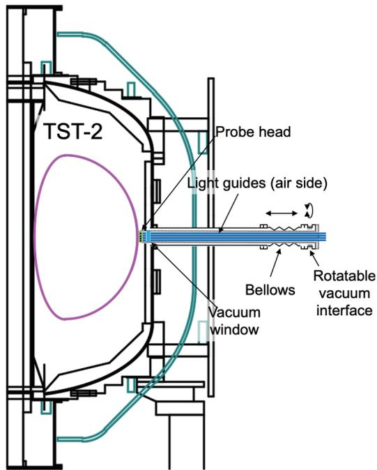
Fig. 8 Schematic drawing of an installation of energetic electron probe.
