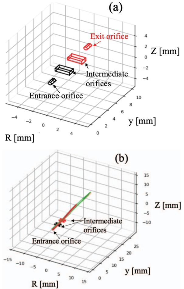
Fig. 3 Orifices to specify electron orbits. (b) Orbits specified by the orifices.
