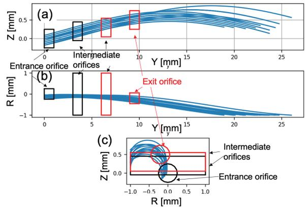
Fig. 5 Orbits specified by the orifices. Arranged in the same way as Fig. 4. In this case, the energy and pitch angle of injected electrons are 50 keV and 4 degrees.
