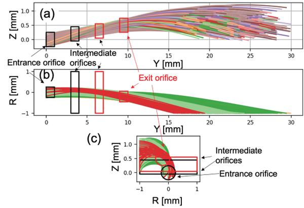
Fig. 4 Orifices and orbits specified by the orifices. (a) They are projected on  $YZ$  surface, (b) on  $YR$  surface, (b) on  $RZ$  surface.
