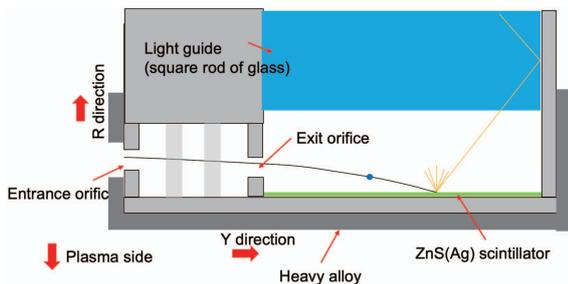
Fig. 7 Schematic drawing of a cross-section of one channel on the YR surface.
