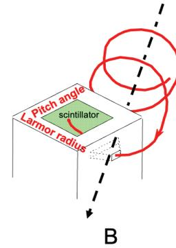
Fig. 1 Schematic drawing of the scintillator-based fast ion loss detector (LIP).
