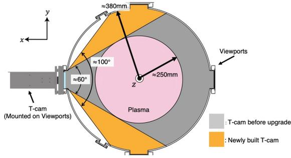
Fig. 6 Comparison of the field of view of newly built T-cam and the T-cam before upgrade. The pink circle indicates the typical cross-section of Merged-FRC.
