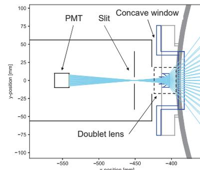
Fig. 4 Arrangement of the T-cam with newly-designed incident optical component.
