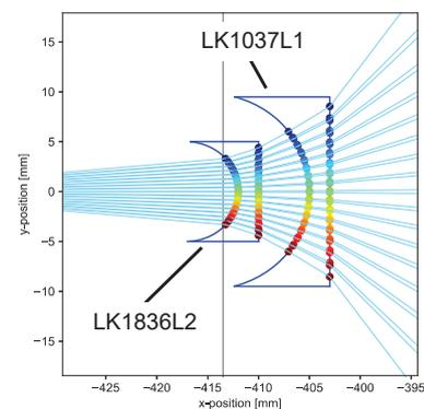
Fig. 5 Ray tracing diagram with lens configuration.
