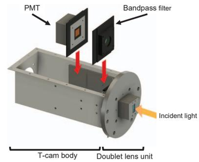
Fig. 3 3D schematic image of the newly-built T-cam.
