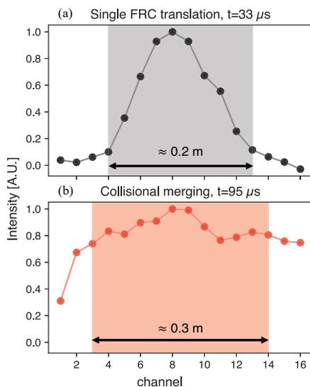
Fig. 2 Radiation profiles of (a) single FRC translation and (b) collisional merging cases captured using the previous T-cam design. The horizontal axis represents channels of multi-anode PMT mounted on T-cam. The gray and red shaded areas indicate FRC size. The edges correspond to the separatrix.
