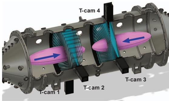
Fig. 1 Arrangement of T-cams on the confinement chamber.
