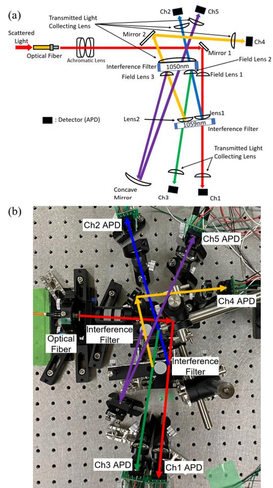
Fig. 3 (a) The schematic of the polychromator system with two angled filters (1059 nm, 1050 nm). (b) The experimental setup of the polychromator system with two angled filters (1059 nm, 1050 nm).
