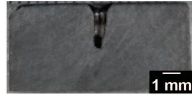
Fig. 8 Graphite target cross section after 10000 pulses.
