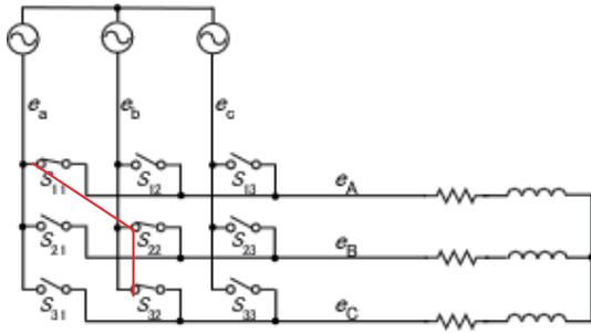
Fig. 2 Direct-type matrix converter. Switches  $S_{11}$ ,  $S_{22}$  and  $S_{32}$  are on. The on switches are connected by the red line, corresponding to the switching configuration (+1) or (1, 2, 2).
