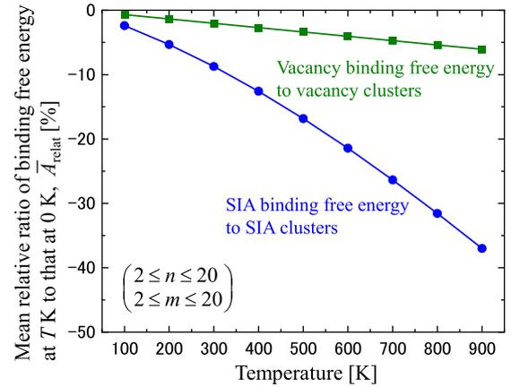
Fig. 2 Temperature dependence of the binding free energy of point defects to small defect clusters in bcc Fe.
