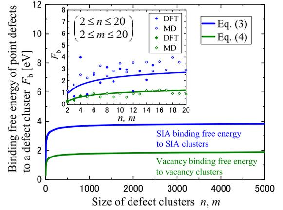
Fig. 1 Size dependence of the binding free energy of point defects to a defect cluster at  $0 \text{ K}$  in bcc Fe.
