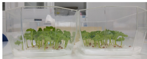
Fig. 8 Growth test of radish-sprout, left: Test group with plasma treated water; right: Control with distilled water.
