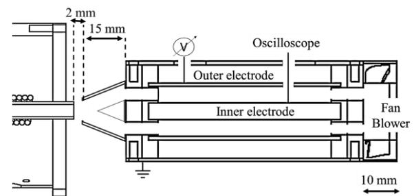
Fig. 3 Schematic diagram of the Gerdien condenser coupled to the atmospheric plasma source.
