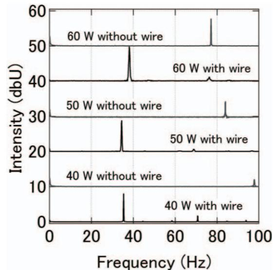
Fig. 8 Fourier transform signal analysis using the Gerdien condenser.
