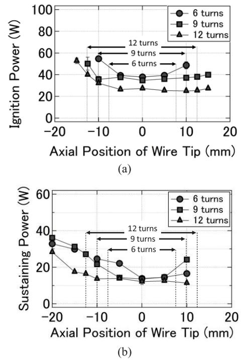
Fig. 5 (a) Ignition power, (b) sustaining power measured when the ignition wire tip position is changed with respect to the midsection of the copper solenoid coil.
