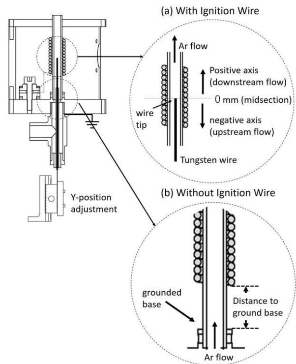
Fig. 2 Schematic diagram of the inductively coupled plasma.
