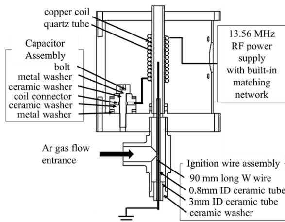
Fig. 1 Schematic diagram of the ion source.
