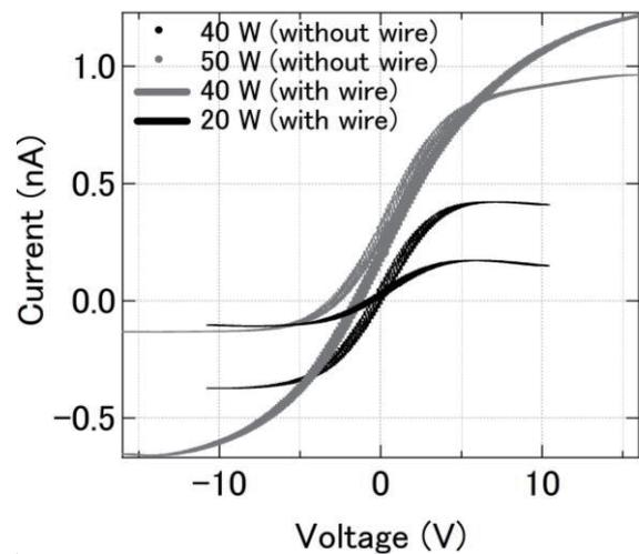
Fig. 6 Typical *I-V* measurements of the Gerdien condenser from the ICP with and without the ignition wire.
