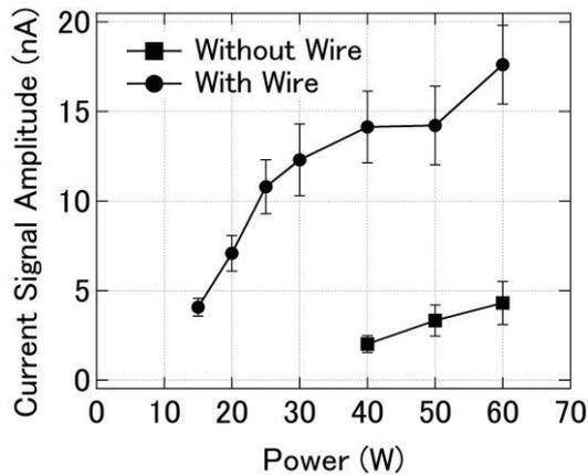
Fig. 7 Amplitude measurements of the temporal change in ion current saturation with +5 V constantly applied voltage to the Gerdien condenser.
