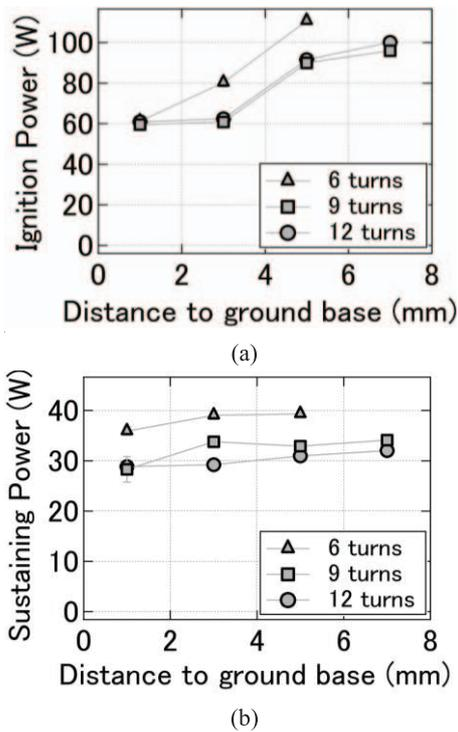
Fig. 4 (a) Ignition power and (b) sustaining power measured when the coil position to the ground base is changed.
