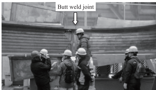
Fig. 8 Butt joint of the top of the TF coil case.
