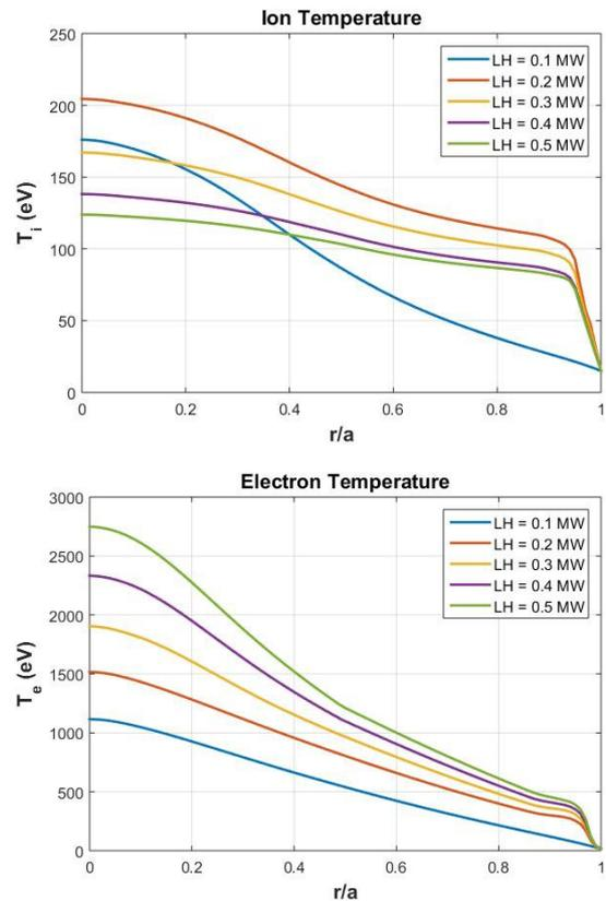
Fig. 8 Ion and electron temperatures as functions of normalized minor radius defined by toroidal flux of plasma when  $I_p = 100$  kA,  $B_\phi = 1.5$  T and LH power was varied.
