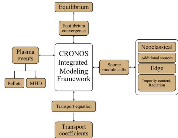
Fig. 1 Global CRONOS workflow with the main sophisticated physics modules around the core transport equation solver.
