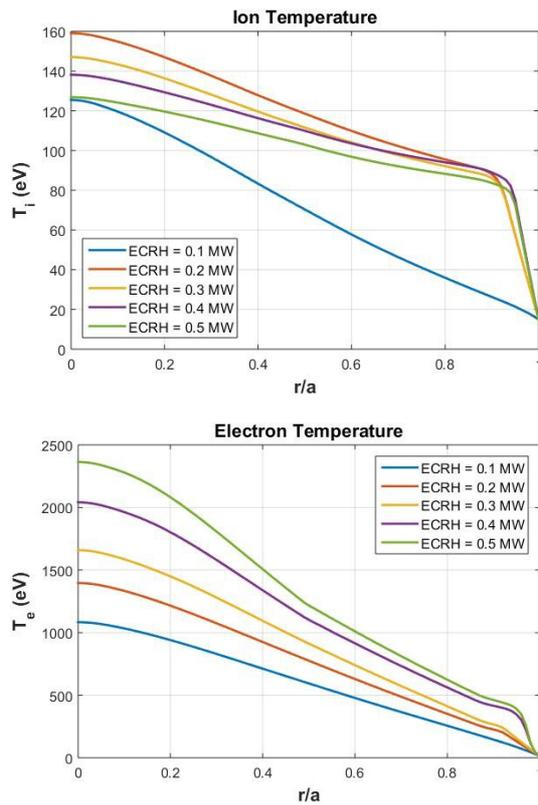
Fig. 6 Ion and electron temperatures as functions of normalized minor radius defined by toroidal flux of plasma when  $I_p = 100$  kA,  $B_\phi = 1.5$  T and ECRH power was varied.
