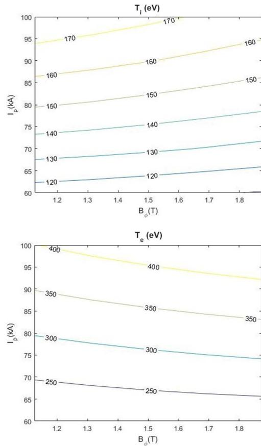
Fig. 3 Contour plots of central ion (top) and electron (bottom) temperatures at various plasma currents and toroidal magnetic fields.
