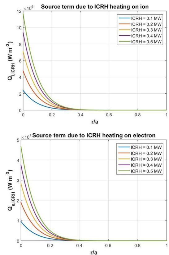
Fig. 5 Source term due to ICRH heating on ion and electron.
