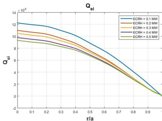
Fig. 7 The electron-ion energy exchange in ECRH power.
