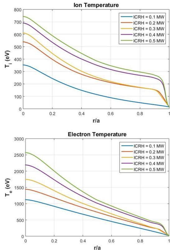
Fig. 4 Ion and electron temperatures as functions of normalized minor radius defined by toroidal flux of plasma when  $I_p = 100$  kA,  $B_\phi = 1.5$  T and ICRH power was varied.
