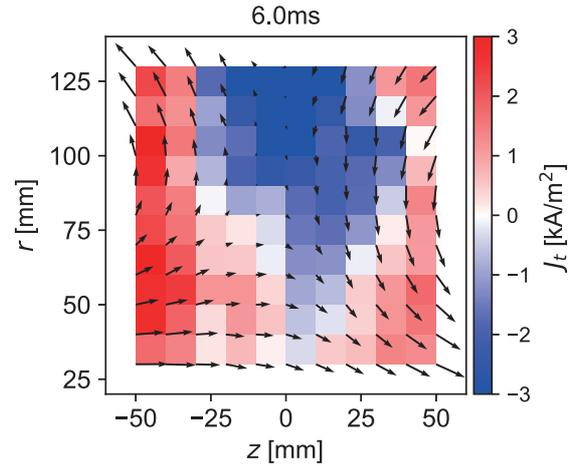
Fig. 4 Profiles of poloidal magnetic field and toroidal current density derived from magnetic sensor signals. Arrows show the strength and direction of magnetic field, and color shows toroidal current density. In contrast to ordinary RMF-FRC plasmas, the reversed current layer was steadily observed around the midplane ( $z = 0$  m).
