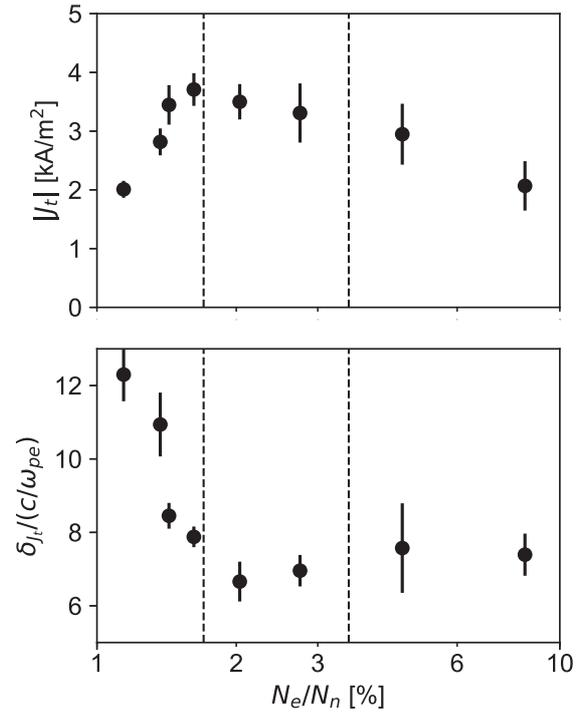
Fig. 7 Dependencies of maximum toroidal reversed current density (top), and the current sheet thickness normalized to electron skin depth (bottom) on ionization degree.
