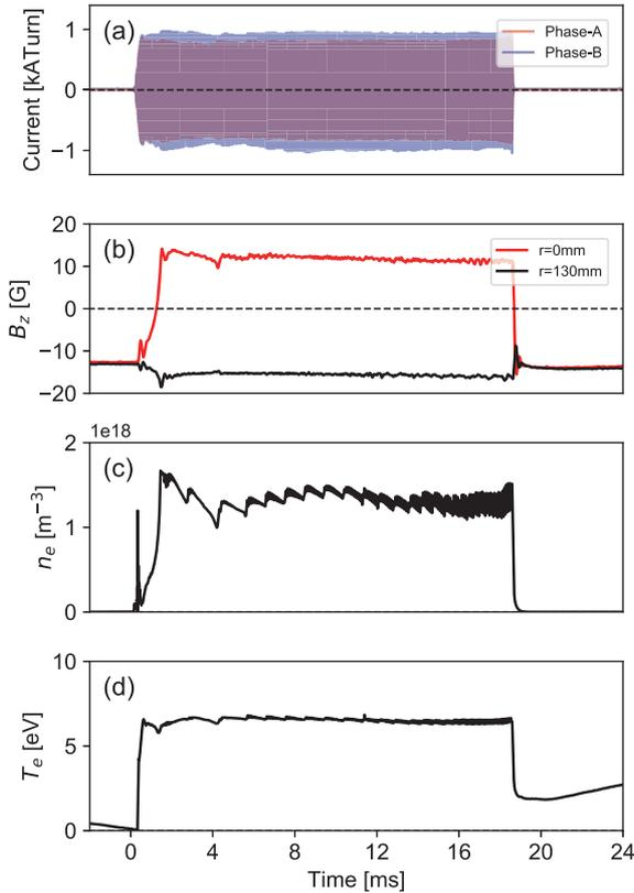
Fig. 3 Time evolution of (a) RMF antenna current, (b) axial magnetic field  $B_z$  at  $r = 0$  mm and  $r = 130$  mm,  $z = -200$  mm, (c) electron density  $n_e$  at  $r = 50$  mm,  $z = -200$  mm, (d) electron temperature  $T_e$  at  $r = 50$  mm,  $z = -200$  mm in the case of helium discharge with the fill-gas pressure of 0.6 mTorr.
