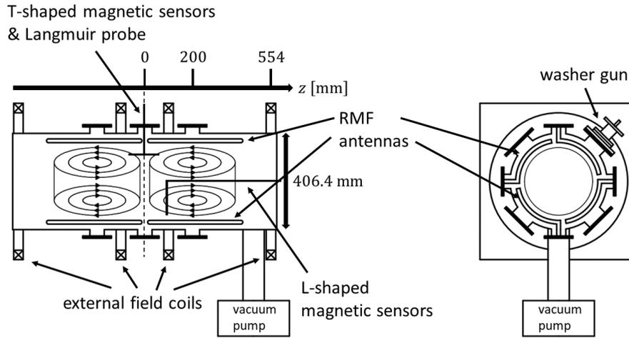
Fig. 1 Schematic view of the experimental device. Axial cross section (left) and radial cross section (right). Four 9-turn RMF antennas are installed on the left and right inside the vessel. Magnetic reconnection occurs on the midplane ( $z = 0$  m), between the two FRC plasmas formed by RMF.
