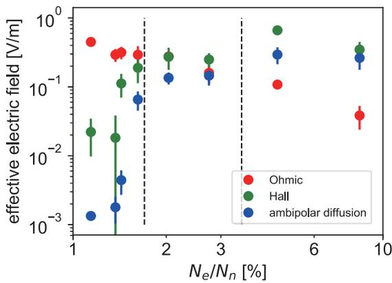
Fig. 6 Dependencies of the toroidal components of the Ohmic term  $-\eta J_t$ , the Hall term  $-(\mathbf{J} \times \mathbf{B}/e n_e)_t$ , and the ambipolar diffusion term  $[(\mathbf{J} \times \mathbf{B}) \times \mathbf{B}/v_{in} m_i n_i]_t$  of the induction equation inside the current layer ( $r = 100$  mm,  $z = 20$  mm) on ionization degree.
