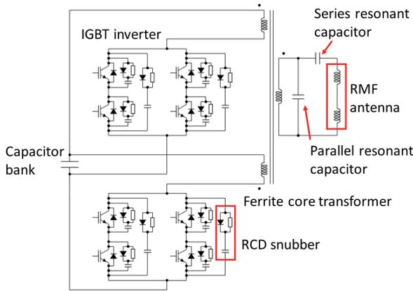
Fig. 2 Circuit diagram of the RMF power supply circuit composed of a capacitor bank, a push-pull inverter circuit, a ferrite core transformers, and a series resonant circuit.
