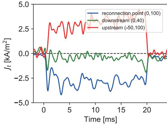
Fig. 5 Time evolution of toroidal current density  $J_t$  at the upstream region (red), downstream region (green), and reconnection point (blue). Negative current was maintained for 20 ms at the reconnection point.
