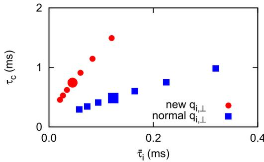
Fig. 5 Particle confinement time  $\tau_c$  as a function of  $\bar{\tau}_i$ ; the new  $q_{i,\perp}$  model (circles) and the normal one (squares). The larger symbols represent the cases with  $\alpha_\tau = 1$ .
