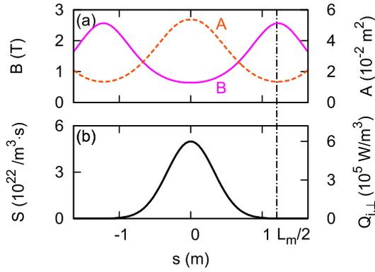
Fig. 1 Parallel-to- $B$  profiles of (a)  $B$  (solid line),  $A$  (broken line), (b)  $S$  and  $Q_{i,\perp}$ . The vertical chain line represents the position of the local maximum of  $B$  ( $s = L_m/2$ ).
