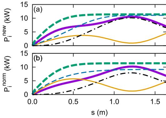
Fig. 4 Power fluxes,  $P_{i,\perp}^{\text{tot}}$  (thick solid),  $P_{i,\parallel}^{\text{tot}}$  (thin solid),  $P_{i,\perp}^{\text{Q}}$  (thick broken),  $P_{i,\text{rx}}^{\perp\rightarrow\parallel}$  (thin broken) and  $P_{i,\text{mirr}}^{\parallel\rightarrow\perp}$  (thin chain lines), with (a) the new  $q_{i,\perp}$  model and (b) the normal one.
