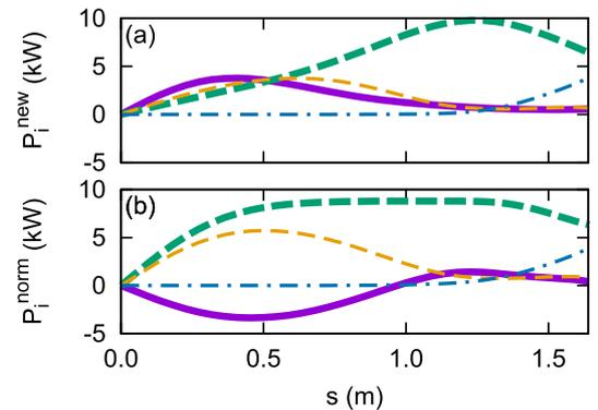
Fig. 3 Power fluxes,  $P_{i,\perp}^{\text{cond}}$  (thick solid),  $P_{i,\perp}^{\text{conv}}$  (thick broken),  $P_{i,\parallel}^{\text{conv,int}}$  (thin broken) and  $P_{i,\parallel}^{\text{conv,flow}}$  (thin chain lines), with (a) the new  $q_{i,\perp}$  model and (b) the normal one.
