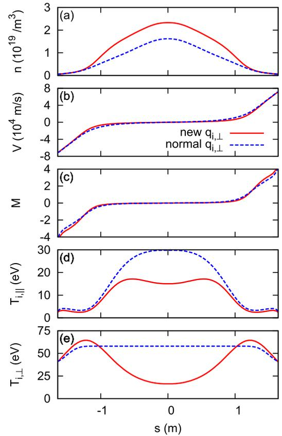
Fig. 2 Parallel-to- $B$  profiles of plasma parameters between the new  $q_{i,\perp}$  model (solid lines) and the normal one (broken lines); (a)  $n$ , (b)  $V$ , (c)  $M$  (d)  $T_{i,\parallel}$  and (e)  $T_{i,\perp}$ .
