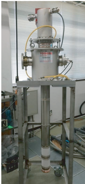
Fig. 3 Photograph of the 303 GHz gyrotron. A Gaussian-like beam is radiated through the vacuum window located at the left hand side.
