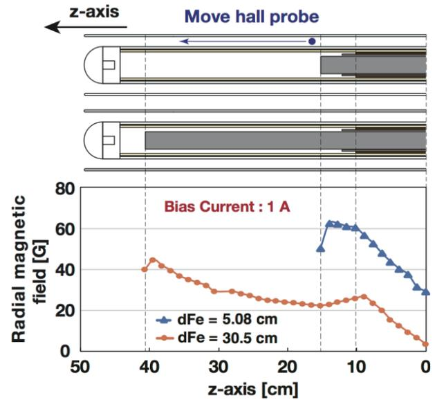
Fig. 2 Axial distribution of radial magnetic field  $B_r$  measured by a hall probe at the middle of the gap between electrodes.
