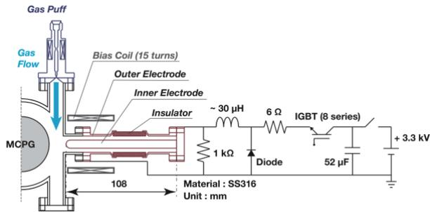
Fig. 3 The diagram of the experimental setup with the discharge circuit. This cross-section corresponds to the dashed line in Fig. 1.
