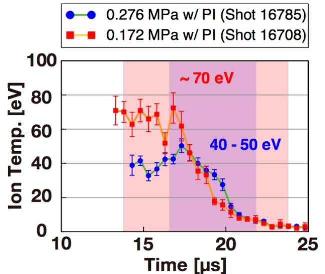
Fig. 6 Typical ion temperature estimated by Doppler broadening of C III line at 0.276 MPa and 0.172 MPa with the PI system. The darkened areas are full width at half maximum (FWHM) at each case in the signal of the collimated fiber at the same cross-section of the spectrometer.
