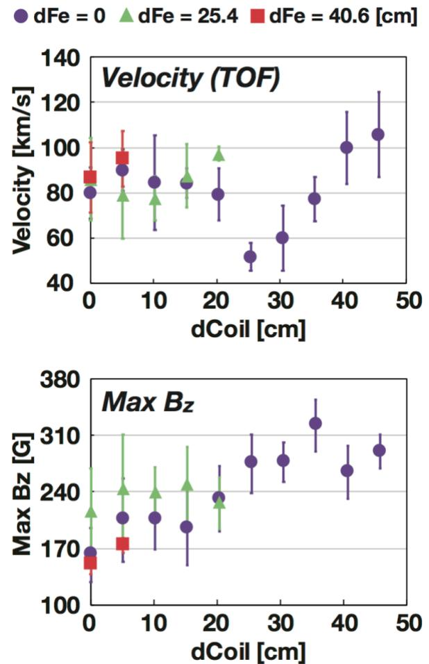
Fig. 4 Dependency of CT parameters on iron-core length ( $dFe$ ) and coil position ( $dCoil$ ) without the PI system.
