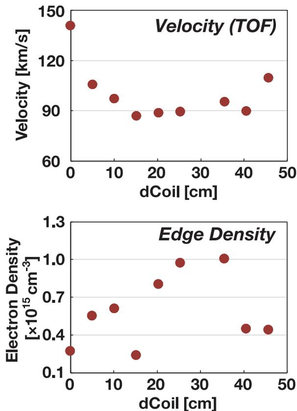
Fig. 5 CT parameters at lower bias current and gas pressure with the PI system.
