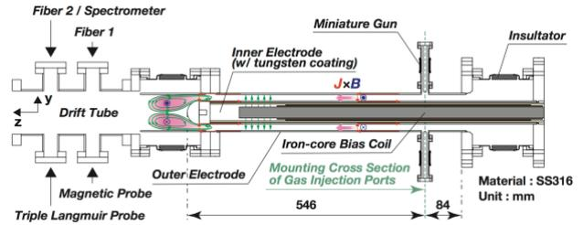
Fig. 1 Schematic drawing of the developed MCPG.
