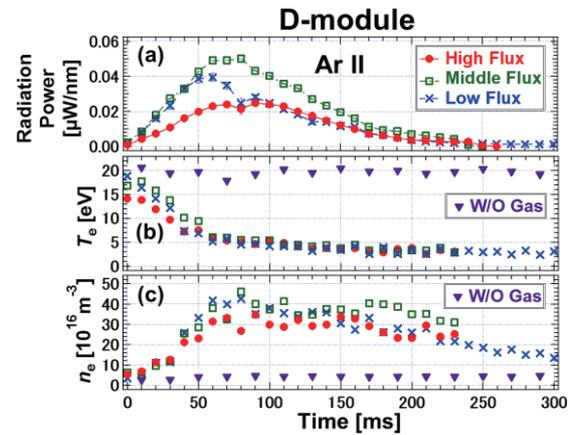
Fig. 3 (a) Ar II (473.59 nm) intensity measured by USB2000+, (b) electron temperature and (c) electron density observed by probe No. 3.
