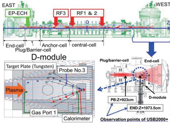
Fig. 1 Schematic view of GAMMA 10/PDX and D-module.
