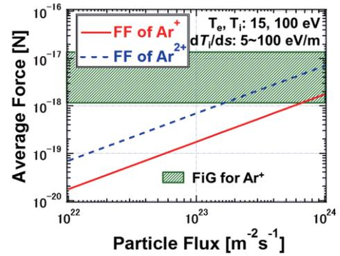
Fig. 8 FF as a function of particle flux and FiG in the range of ion temperature gradient ( $d(kT_i)/ds$ ): 5 ~ 100 eV/m.
