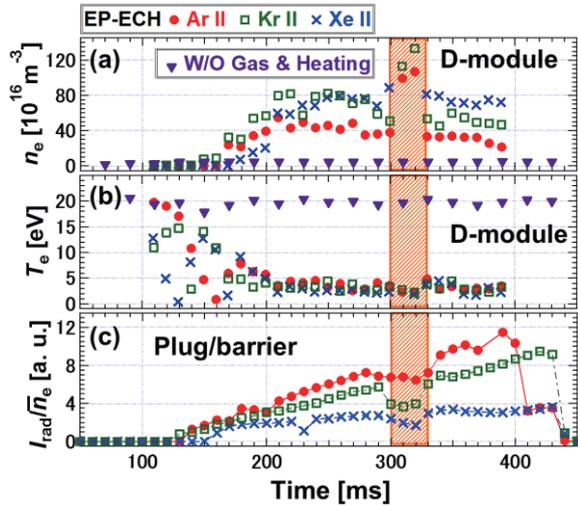
Fig. 7 (a) Electron density and (b) temperature observed by probe No. 3. (c)  $I_{\text{rad}}/\bar{n}_e$  calculated from Eq. (1).
