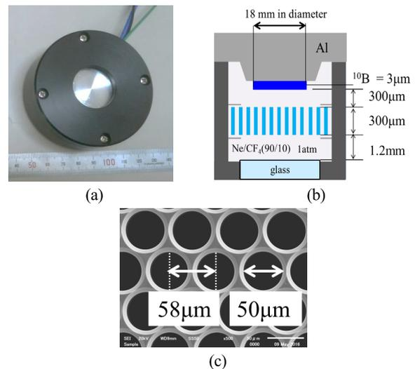
Fig. 2 (a) Sealed-type CP gas detector. (b) Cross-section of the detector comprises a <sup>10</sup>B layer, a CP, and a sealed chamber filled with Ne (90%) + CF<sub>4</sub> (10%) at 1 atm. (c) SEM image of the CP with 50-μm diameter holes and a 58-μm pitch.
