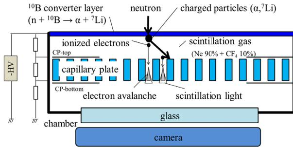
Fig. 1 Schematic view of a CP gas detector for neutron imaging.
