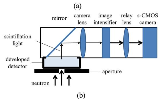
Fig. 3 Experimental setup of the neutron imaging system.
