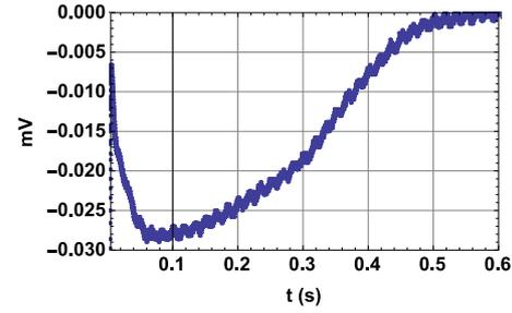
Fig. 3 Faraday cup signal for the case of 6550 particles (6 rotations of the conveyer) at  $1 \text{ M}\Omega$  input impedance.
