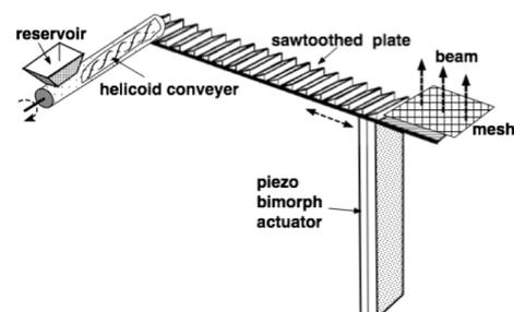
Fig. 1 Illustration of the beam source of highly charged micro-particles.
