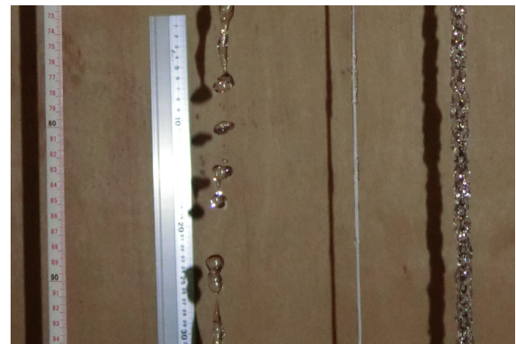
Fig. 2 The photo of a normal jet (left), a sheath jet with a wood pole (center), and a sheath jet with chain (right). The exposure time of this photo was 0.001 s.
