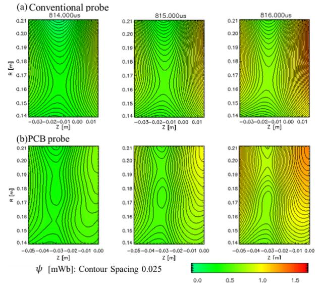
Fig. 2 2D poloidal flux contours of two merging ST plasmas measured by (a) the conventional pickup coil arrays and (b) the new PCB probe arrays.
