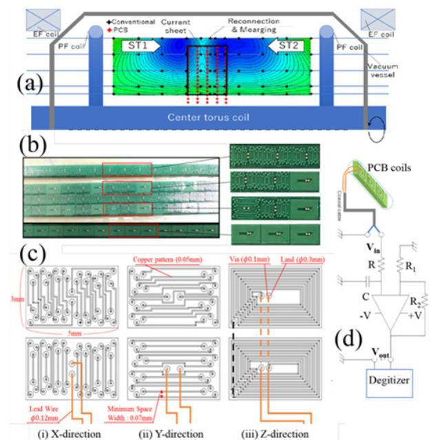
Fig. 1 (a) 2D setup of conventional pickup coils (black crosses) and PCB coils (red crosses) on the  $r$ - $z$  poloidal flux contour of two merging ST plasmas. (b) Four types of PCB probe arrays composed of (c) three coil circuit patterns for  $B_x$ ,  $B_y$ , and  $B_z$ . (d) Integrating and amplifying circuits for each PCB coil for the magnetic field measurement.
