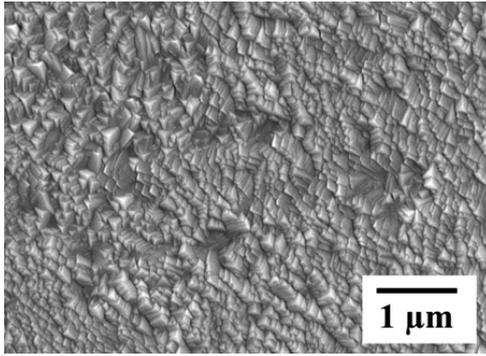
Fig. 2 SEM image of the SP-W coatings surface.
