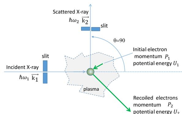
Fig. 1 Measurement scheme of inelastic Compton scattering of plasma.
