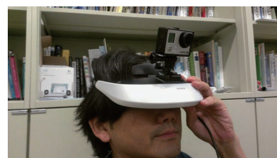
Fig. 2 A head-mounted display (HMD) system.
