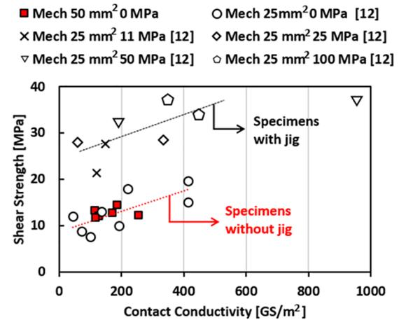
Fig. 6 Shear strength as a function of contact conductivity for mechanical lap-joint of GdBCO CCs at 77 K.
