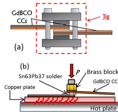
Fig. 1 (a) Mechanical lap-joint fabrication set-up, (b) Soldered lap-joint fabrication set-up.
