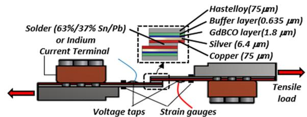
Fig. 2 Experimental set-up of the tensile shear test.
