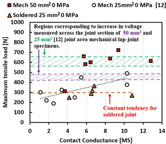
Fig. 3 Maximum tensile load as a function of contact conductance characteristics for mechanical and soldered lap-joint of GdBCO CCs at 77 K.
