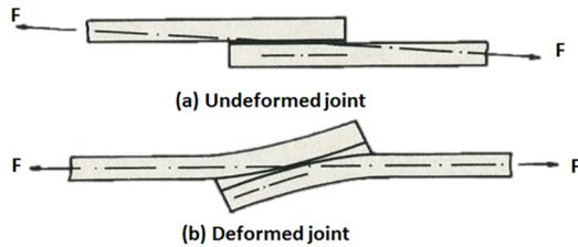
Fig. 7 The Goland and Reissner bending moment factor (geometric illustration) [16].
