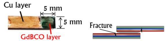
Fig. 5 Picture of one of the soldered lap-joint samples after tensile shear test was performed.
