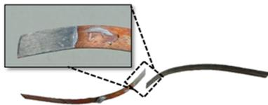
Fig. 4 Mechanical lap-joint sample with a joint area of 50 mm<sup>2</sup> after being pulled apart.
