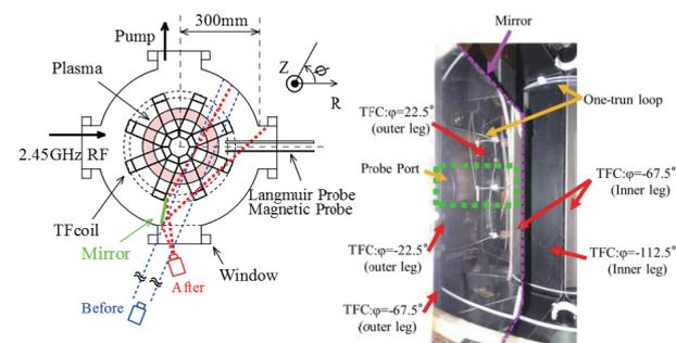
Fig. 2 (Left) Top view of high-speed camera sightlines. (Right) Photograph of the view in the tangential direction.
