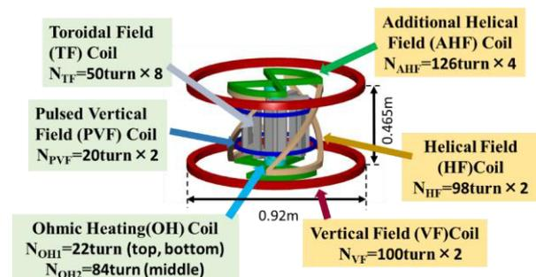
Fig. 1 Coil system of TOKASTAR-2 device.
