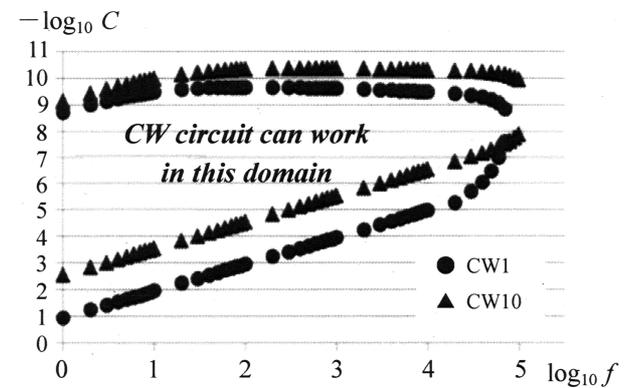
Fig. 4 Frequency of power source and capacity (If combinations of frequency and capacity enter the domain surrounding a plot, the CW circuit can work).
