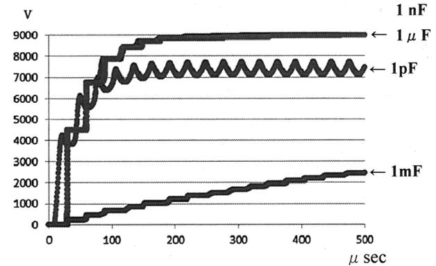
Fig. 3 Capacitance and boost voltage ( $E_0 = 4500$  V,  $f = 35220$  Hz, and  $k = 1$ ).
