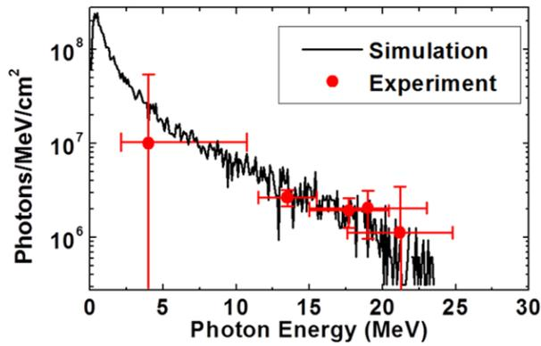
Fig. 4 Result of measurement of X-ray spectrum. Black point shows X-ray spectrum calculated by using PHITS-code [10] (black point). Red point shows experimental data. Cross-talk and full width at half maximum of photo-nuclear reaction cross-section are accounted in the error bars.
