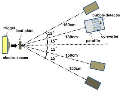
Fig. 3 Experimental configuration of evaluating performance.
