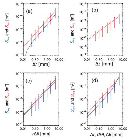
Fig. 2  $S_{x-y}$  and  $S_{x-z}$  of the two layer winding, where,  $\Delta r$ ,  $\Delta z$  and  $r\Delta\theta$  are errors in each direction.
