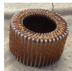
Fig. 4 Eight-layer Rogowski coil: Outer diameter = 20 mm; inner diameter = 12 mm; thickness = 12 mm; number of turn 360; sensitivity =  $5.0 \times 10^{-7}$  Vs/A; and thickness of the cable = 0.12 mm.
