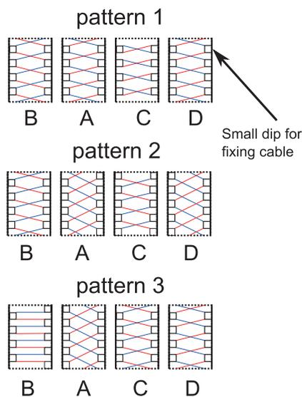
Fig. 3 The three fabricated patterns are shown. Surfaces A, B, C and D denote the four surfaces of the rectangular cross section (see Fig. 1). They are the top, inner, bottom, and outer sides, respectively.
