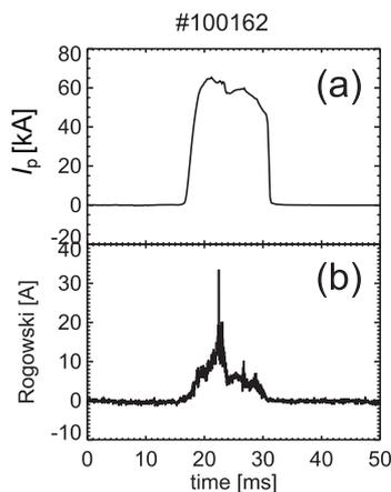
Fig. 5 The time evolution of the plasma current (a) and the local current measured by the Rogowski coil (b).
