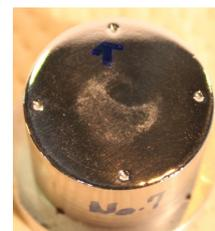
Fig. 2 Test piece surface after cyclic loading and 60 s of vacuum cleaning.
