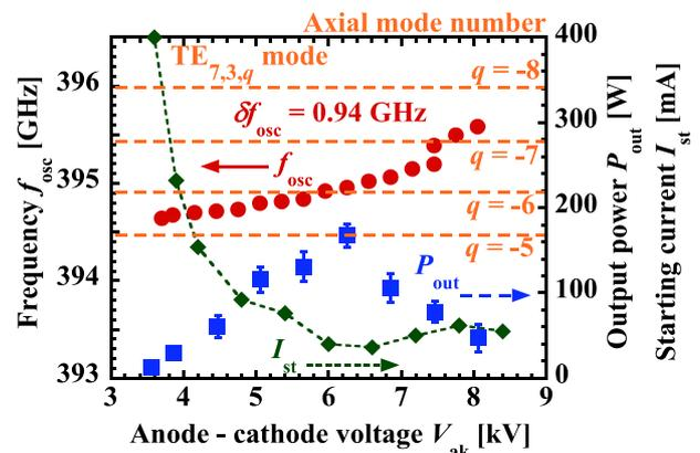
Fig. 3 Anode-cathode voltage dependence of the oscillation frequency, output power, and starting current.
