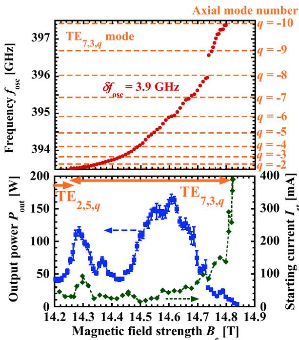
Fig. 2 Magnetic field dependence of the oscillation frequency, output power, and starting current.
