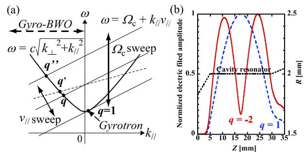
Fig. 1 (a) Dispersion relation of Gyro-BWO oscillation. (b) Schematic view of the axial mode in the cavity resonator.
