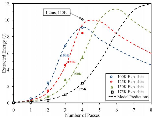
Fig. 4 Predicted output energy of the DiPOLE amplifier for 8 passes along with the experimental values measured for up to 4 passes at different temperatures for 1 Hz operation and 1 ms pump pulse duration.
