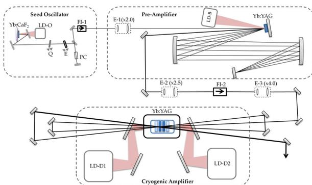
Fig. 2 Schematic diagram of the DiPOLE system.
