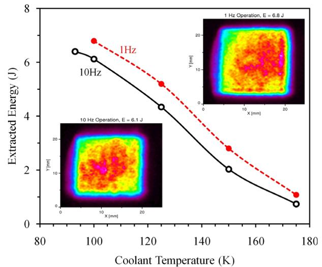
Fig. 6 Extracted energy from the main amplifier at 1 Hz and 10 Hz pulse repetition rates for a 3-pass extraction setup at different temperatures and for fixed pump pulse duration of 1 ms. Inserted are the typical beam profiles for 1 Hz and 10 Hz after the main amplification stage.
