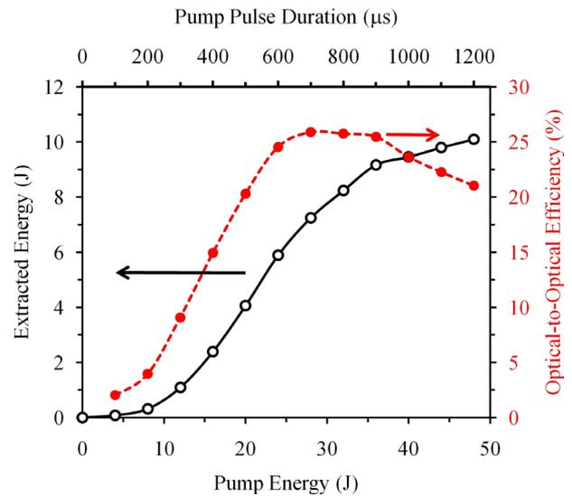
Fig. 5 Extracted pulse energy (solid line) and  $\eta_{o-o}$  (dotted line) of the DiPOLE amplifier for up to 1.2 ms pump pulse duration at 1 Hz, 4-passes and 115 K coolant temperature.
