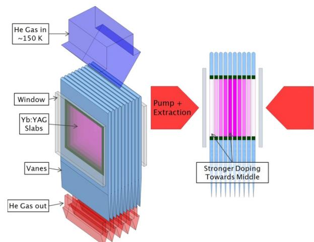
Fig. 1 Illustration of kJ-class amplifier concept: isometric (left) and side view (right).
