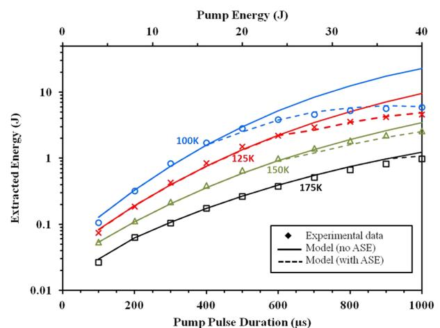
Fig. 3 Extracted energy as a function of pump pulse duration measured at different temperatures for 1 Hz operation in a 3-pass configuration.
