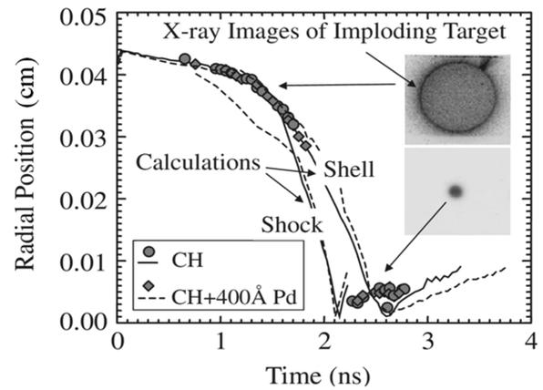
Fig. 9 Implosion trajectory simulated with FASTrad3D agrees with the measurements [9].
