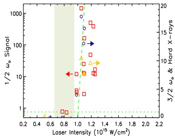
Fig. 10 Measurements are consistent with the simple threshold formula (shaded region) giving higher LPI thresholds for KrF lasers than for 351 nm lasers.
