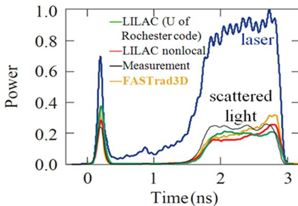
Fig. 8 Measurements of scattered light from Ref [7] simulated by University of Rochester’s code and NRL’s FASTrad3D code.
