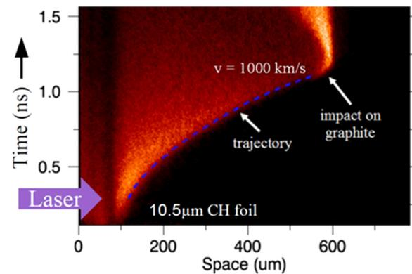
Fig. 6 Side-on x-ray image of an accelerating 10.5  $\mu\text{m}$  CH target. The trajectory traced from the image is overlaid as a dashed line. The impact on a stationary foil marked by bright emission is clearly visible.
