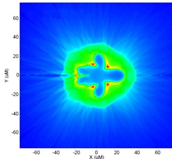
Fig. 3 Density image of a 2D high resolution ( $l = 1-256$ ), 521 kJ KrF implosion with shock ignition at the time of peak  $\rho R$  resulting in a gain of 102 (1D gain is 142). The simulation includes outer and inner surface roughness and ISI laser imprint.
