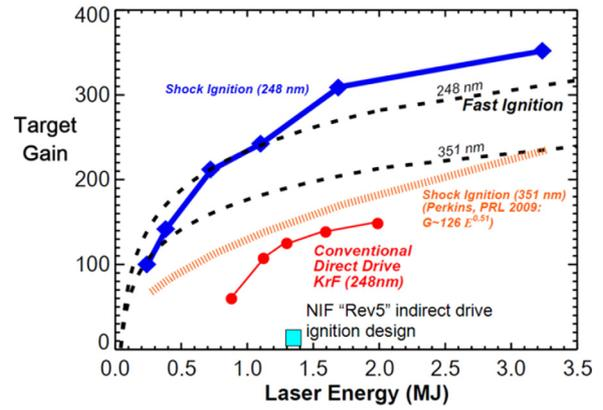
Fig. 2 Shock ignition gain is comparable to fast ignition. Fast ignition curves are based on Ref [3]. 351 nm shock ignition curve is based on Ref [4].
