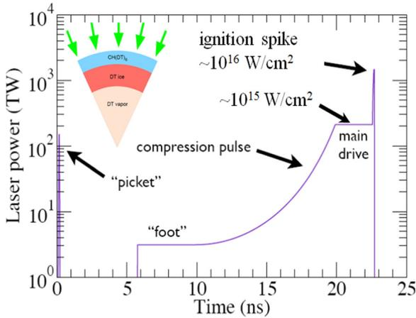
Fig. 1 Shock ignition pulse shape. Inset shows a sector of the pellet with layers: DT-wicked CH foam + DT ice + DT vapor.
