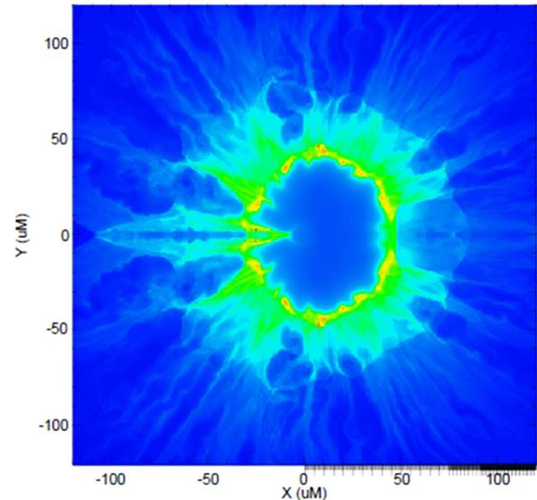
Fig. 5 Increasing initial aspect ratio too far can lead to target failure due to hydrodynamic instability: this aspect ratio 6.2 pellet fails to ignite.
