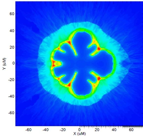
Fig. 4 A higher aspect ratio (3.7), 529 kJ KrF implosion with shock ignition resulting in a gain of 136. The simulation includes outer and inner surface roughness and ISI laser imprint.
