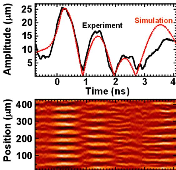
Fig. 7 Top: experimental (solid) and simulated (dotted line) time histories of the areal mass modulation amplitude in a 125 μm thick target with a 45 μm wavelength ripple. Bottom: areal mass perturbations in the range of 22 to 50 μm obtained from an x-ray streak radiograph of the target.
