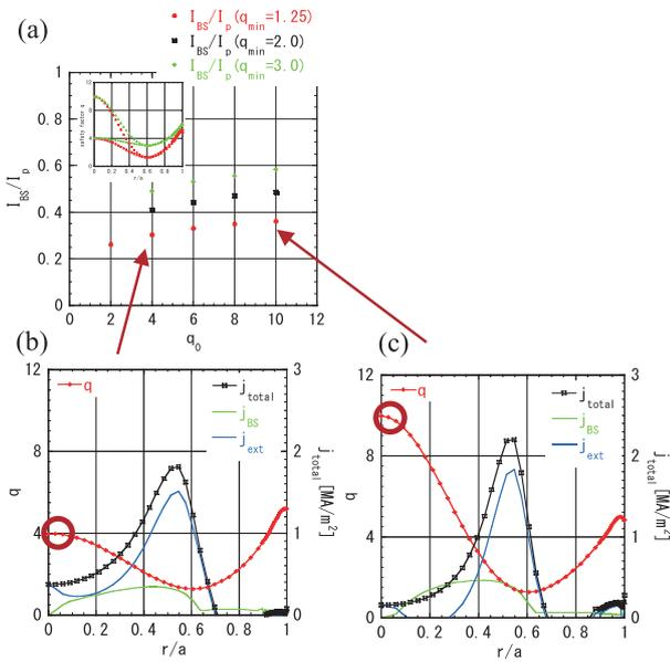
Fig. 4 Effects of changing  $q_0$ . (a) Dependence of (a) Dependence of  $I_{BS}/I_p$  on  $q_0$ . (b) Radial profiles of  $q$ ,  $j_{total}$ ,  $j_{bs}$ , and  $j_{ext}$  for  $q_0 = 4.0$ . (c) Radial profiles for  $q_0 = 10.0$ .
