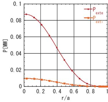
Fig. 2 Profiles of external electron heating power  $P_{\text{exte}}$  and ion heating power  $P_{\text{exti}}$ .
