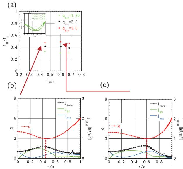
Fig. 6 Effects of changing  $r_{qmin}$ . (a) Dependence of  $I_{BS}/I_p$  on  $r_{qmin}$ . (b) Radial profiles of  $q$ ,  $j_{total}$ ,  $j_{bs}$ , and  $j_{ext}$  for  $r_{qmin} = 0.45$ . (c) Radial profiles for  $r_{qmin} = 0.6$ .
