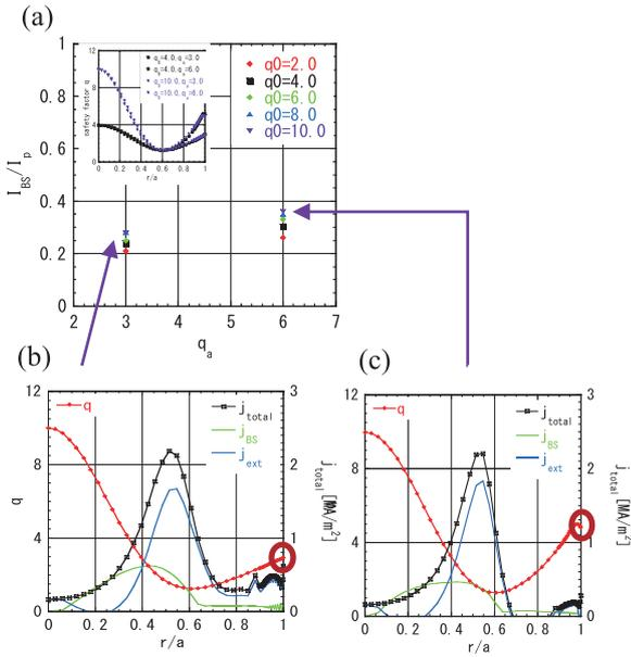
Fig. 3 Effects of changing  $q_a$ . (a) Dependence of  $I_{BS}/I_p$  on  $q_a$  value. (b) Radial profiles for  $q_a = 3.0$ . (c) Radial profiles for  $q_a = 6.0$ . Radial profiles are for safety factor  $q$ , total current density  $j_{total}$ , bootstrap current density  $j_{bs}$ , and external current density  $j_{ext}$ .
