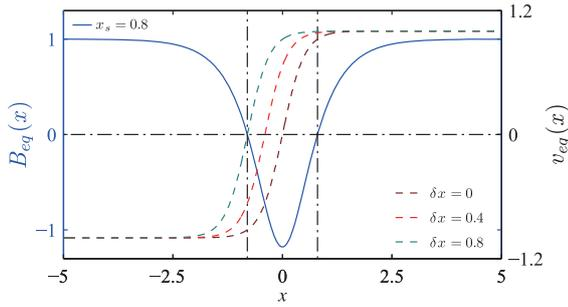
Fig. 1 Equilibrium magnetic field  $B_{\text{eq}}(x)$  with  $x_s = 0.8$  (solid curves) and shear flow profiles  $v_{\text{eq}}(x) = v_0 \tanh(\kappa(x + \delta x))$  with  $\delta x = \{0, 0.4, 0.8\}$  (dashed curves).
