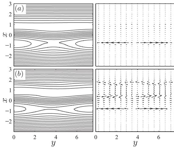
Fig. 4 The island structures (left panel) and corresponding plasma flow patterns (right panel) for different flow amplitude (a)  $v_0 = 0.1$ , (b)  $v_0 = 0.4$ .
