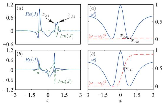
Fig. 5 Radial structures of the perturbed current of the DTM ( $J = \nabla_{\perp}^2 \psi$ ) with negative frequency (left panel) and the corresponding Alfvén resonance condition (right panel) (a)  $v_0 = 0.1$ , (b)  $v_0 = 0.6$ .
