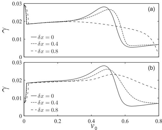
Fig. 7 Growth rates of the DTMs as a function of flow amplitude  $v_0$  for  $\delta x = \{0, 0.4, 0.8\}$ .
