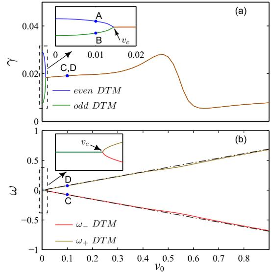
Fig. 2 Linear growth rates (a) and real frequencies (b) of the even and odd DTMs as a function of the flow amplitude  $v_0$  for  $\delta x = 0$ . The dot-dashed lines are reference lines in terms of the Doppler shift frequency  $\omega = kv(\pm x_s)$ .
