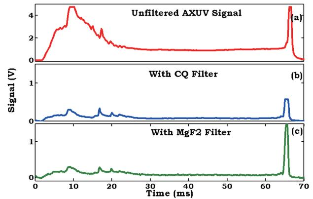
Fig. 5 Signal in the three bolometers:  $P_B$  (a),  $P_{MgF}$  (b) and  $P_{CQ}$  (c).
