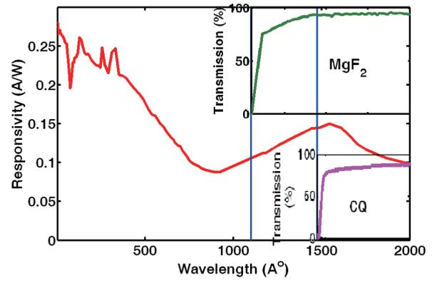
Fig. 2 Filtered AXUV Bolometer Response: Two filters viz. Magnesium Fluoride ( $\text{MgF}_2$ ) and Cultured Quartz (CQ) is used in front of the bolometers.
