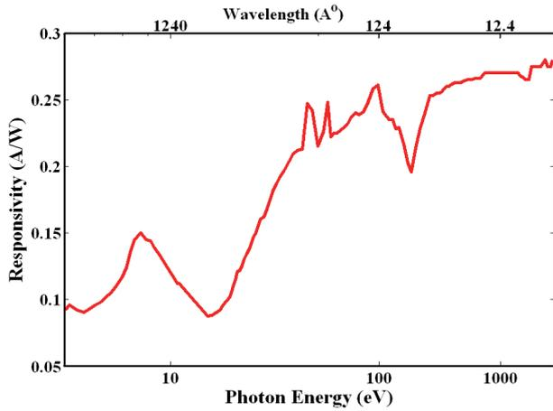
Fig. 1 Responsivity Curve for AXUV Bolometer.
