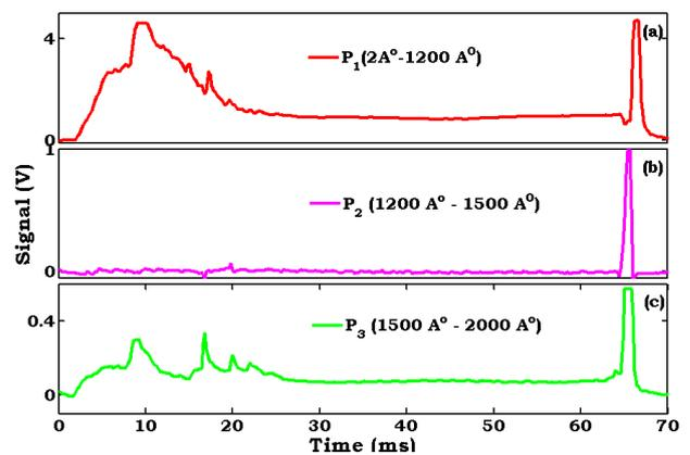
Fig. 6 Radiation signals  $P_1$ ,  $P_2$  and  $P_3$  for a normal ADITYA discharge.
