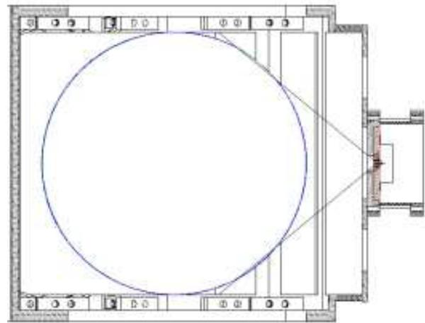
Fig. 3 Bolometer Field of view.
